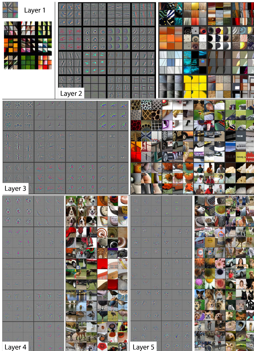
Figure 2.13: Top single strongest activations for a given feature map projected down to pixel space using the approach of [NHH15], showing the hierarchical nature of the features in the network. Layer 2 responds to corners and other edge/color conjunctions. Layer 3 has more complex invariances, capturing similar textures, Layer 4 is more class-specific, Layer 5 shows entire objects with significant pose variation. Image reproduced from [NHH15].
